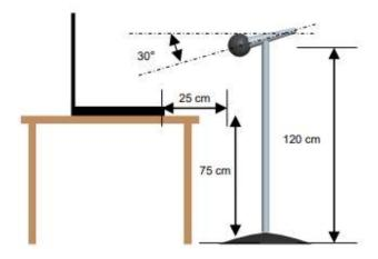
4-4. For B phase test, we determine the fan RPM to meet THTF acoustic SPEC in front side sound pressure.
