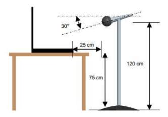
4-4.For B phase test, we determine the fan RPM to meet THTF acoustic SPEC in front side sound pressure.
